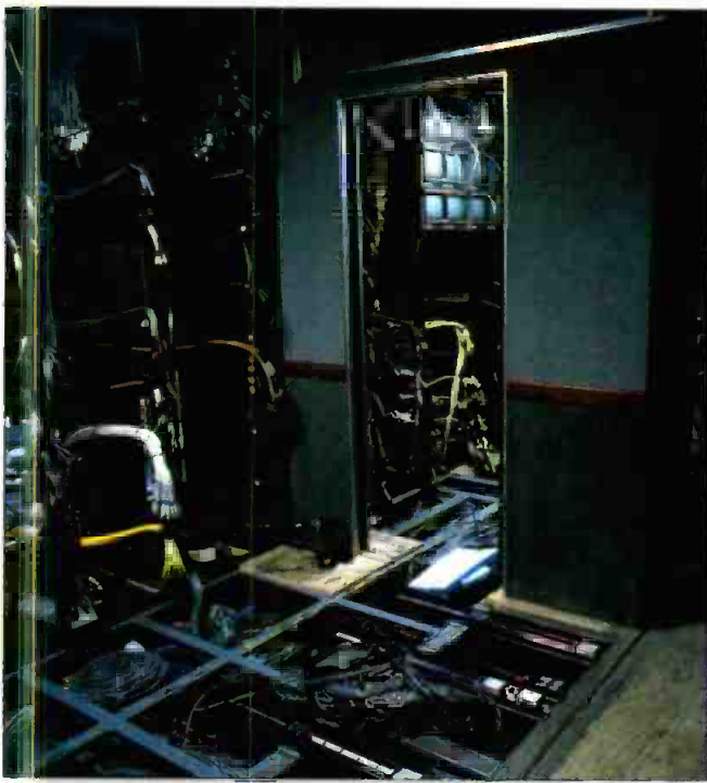
Much of the initial integration work involves getting the correct cables to the proper locations. Note the heavy-gauge welded cross members in the floor. Bolted construction will not stand up to the rigors of road work. (Photo credit: Concept: Benson and Rice)
